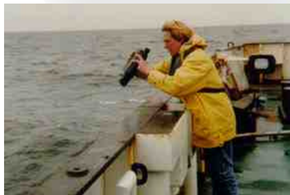
Measurement of water colour is made at sea using a hand-held spectroradiometer
