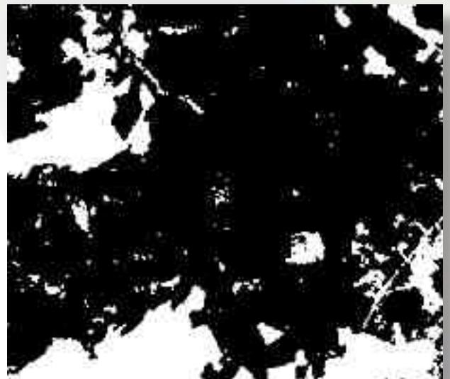
Same mask as in previous figure after modal filtering involving a 3*3 pixel mobile window.
