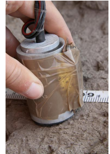
Measuring reflectance spectra on a prepared soil surface
