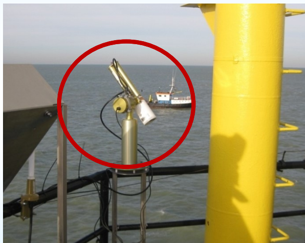
CIMEL-SeaPRISM installed on the Zeebrugge-MOW1 site [courtesy Afdeling Kust]
