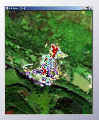
Mine waste of differing mineralogy discriminated using hyperspectral imagery and field spectra (geochemical analysis still needed for identification)
