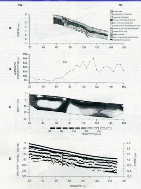
FIG. 7. Site 3. (a) Schematic trench cross-section. (b) Electromagnetic profiling (EM). (c) Electrical tomography. (d) Radar section (50 MHz).
