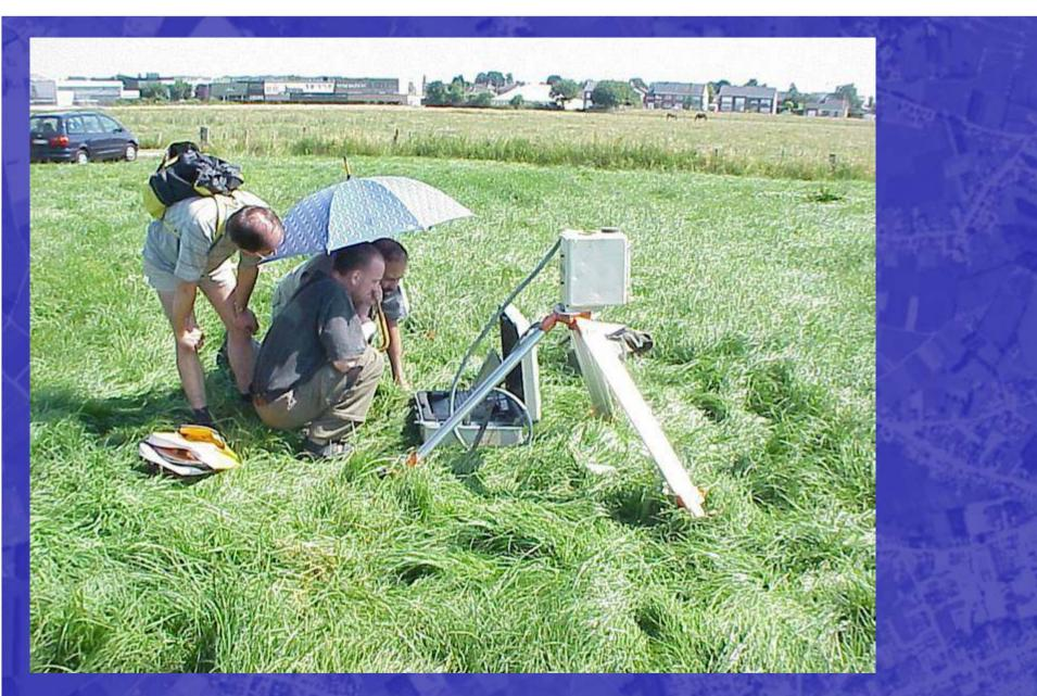
Field spectroradiometric measurements synchronous to the data acquisition, near Houben, Bree
