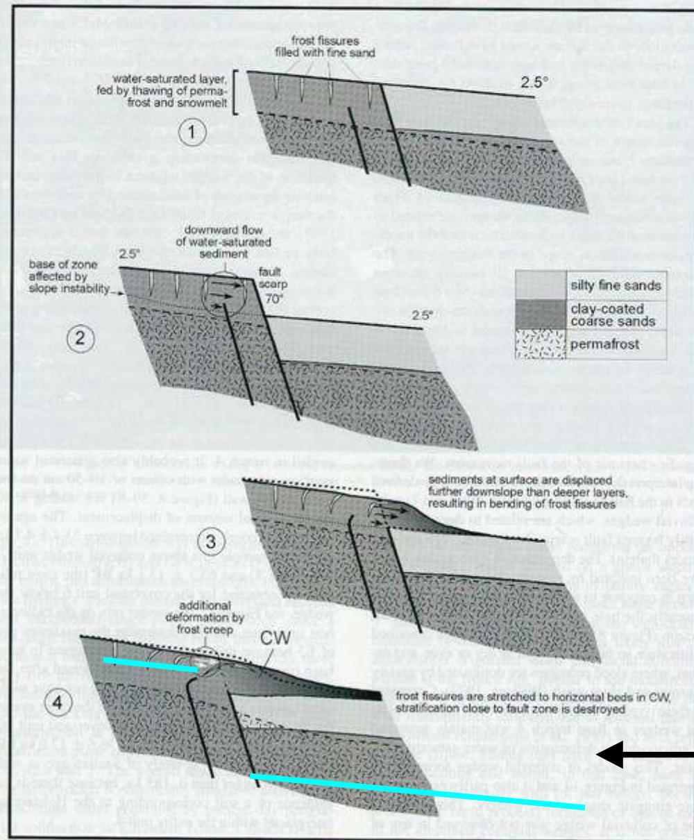
Figure 14. Model for colluvial-wedge development following surface rupture under periglacial conditions at trench site 4. CW = colluvial wedge.
