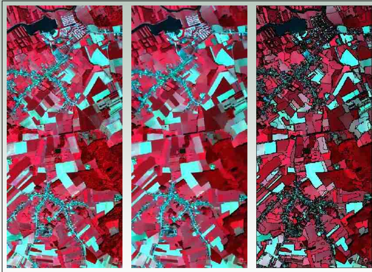
Figure 6.3 A multiscale-based filter is generated using statistical selection of an optimal diffused scale. Left: Original image. Middle: diffused image at the selected scale. Right: segments generated from the diffused image.
