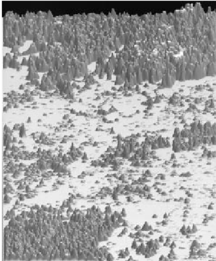
Fig. 9. Three-dimensional representation of the height difference between effective phase scattering centers of the forested areas.
