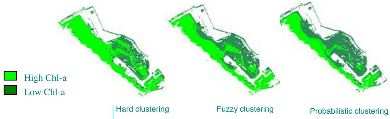
unsupervised classification of a hyperspectral image by different techniques: classifying the IJzermonding in two classes of chl-a
