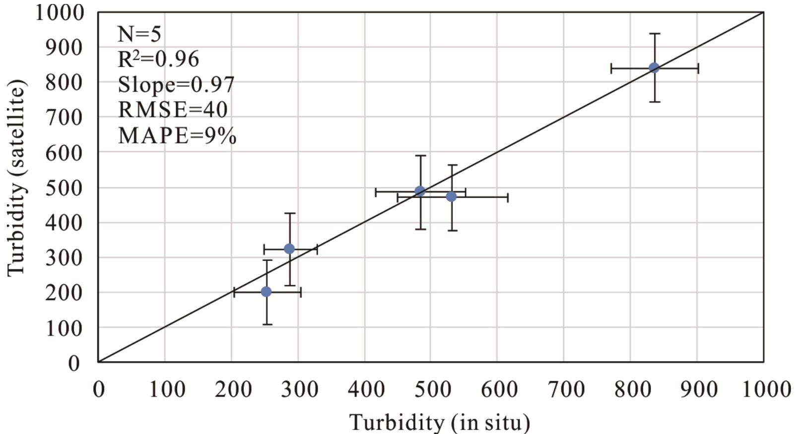
**Match-up comparison of in situ turbidity (NTU) and turbidity derived from reflectance using the Pléiades band of 842 nm**
