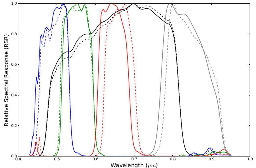
Relative spectral response of the 4 bands on Pléiades-1A (solid lines) and 1B (dashed lines).
