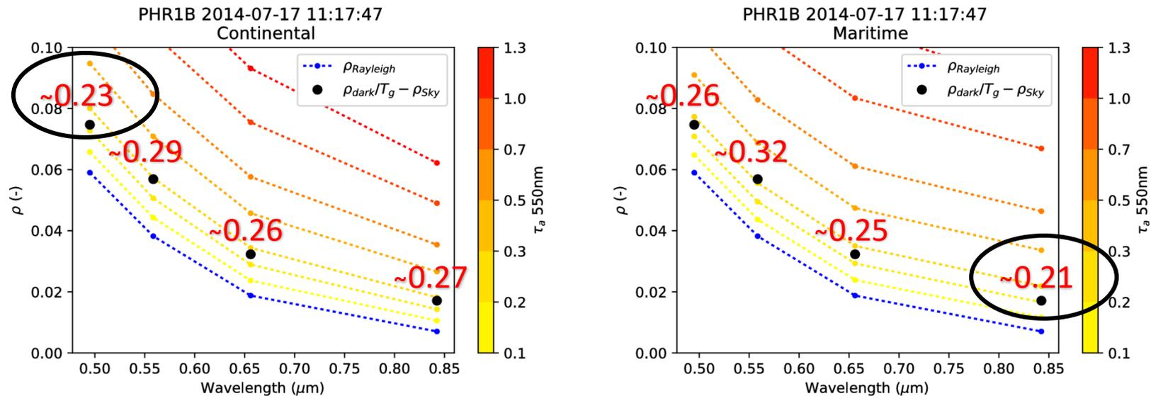
For Pléiades the **model and band combination giving the lowest  $\tau_{a550}$  is selected.** (This criterion avoids negatives values in the  $\rho_{\text{dark}}$  after aerosol correction.)
