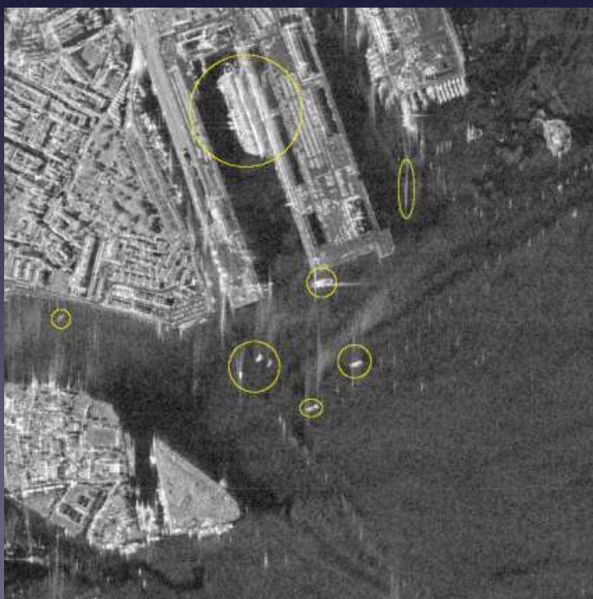
Left: TerraSAR-X Intensity image of the docks of Venice - Right: Corresponding averaged spectral coherence
