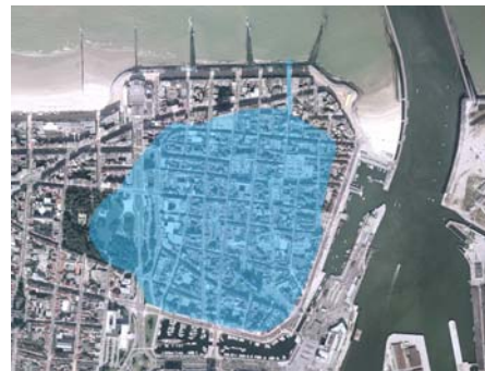
Animation showing the area within the city of Oostende which might possibly flood in case of dike failure.
