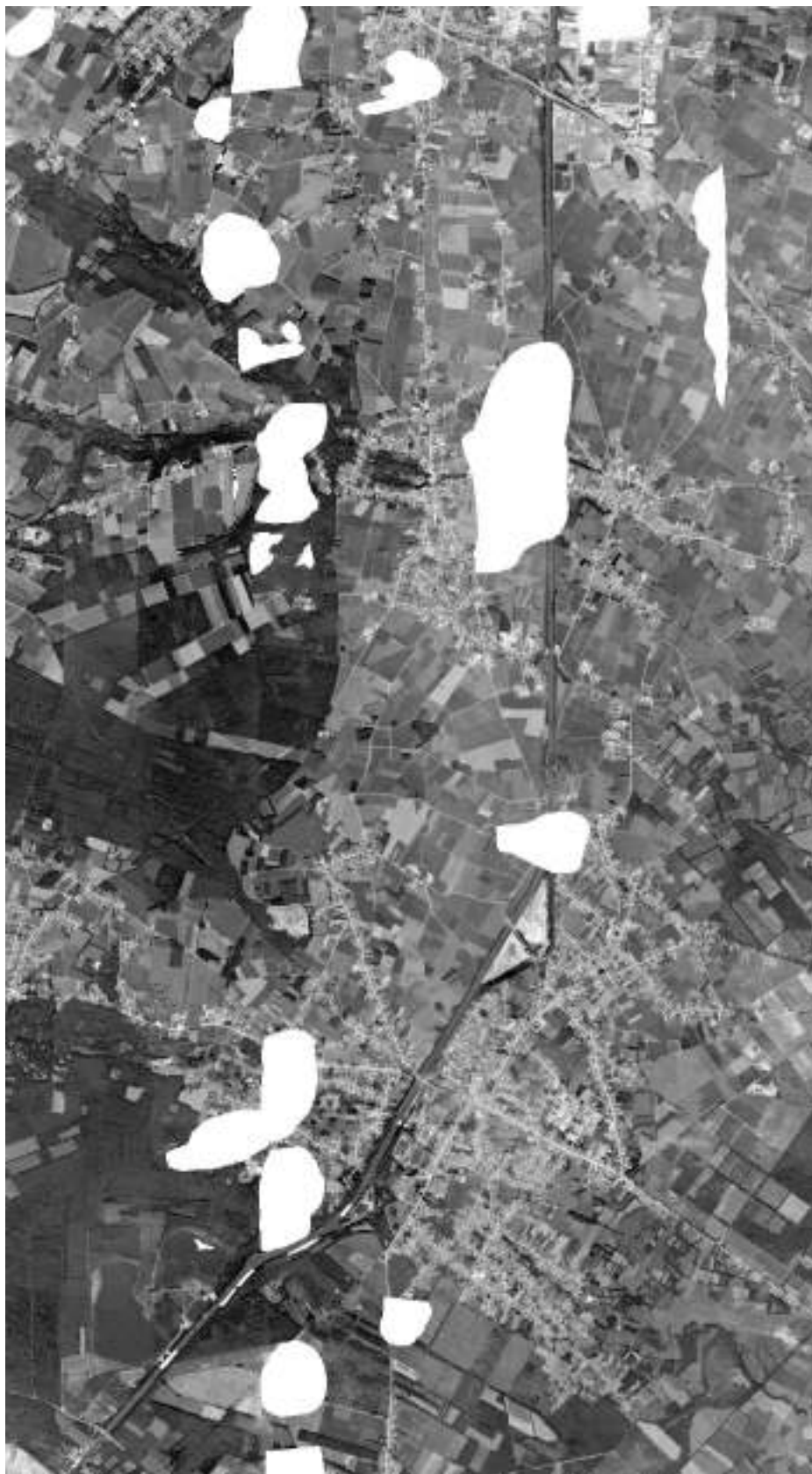
Figure 7. Final mask. The areas in white in the image will be excluded from the data processing.
