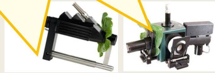
Leaf measurements with leaf clip or integrating sphere (ASD)
