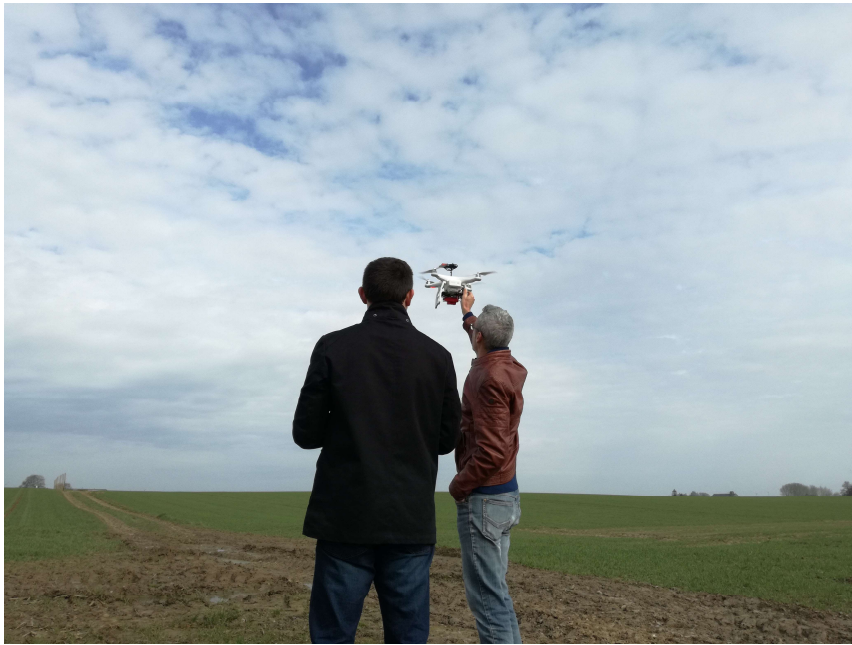
UAV flights with Micasense: 5 cameras : 475 nm - 840 nm : blue, green, red, red-edge, NIR.
